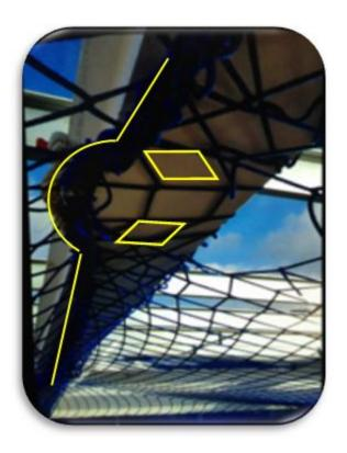
Sometimes we find that in the under-rolling process, and according to the photos displayed, the rolled is formed spinning not equally around its axis, generating that the square meshes lost the parallelism with it and causing that in some of them there were more tensile forces that the rest once the net have been installed so it produces some damages on the net.
